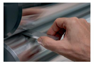
The gap width can be read on the display when you release the wedge.
