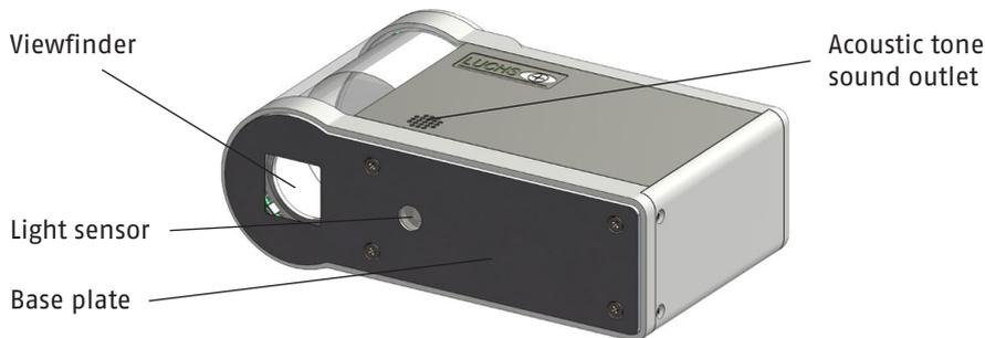
Abb. 2: LUCHS V-Measuring Head, base plate view
