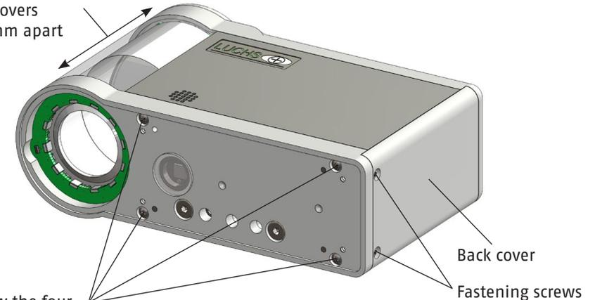
Unscrew the four Phillips head screws 2-2.5 mm
