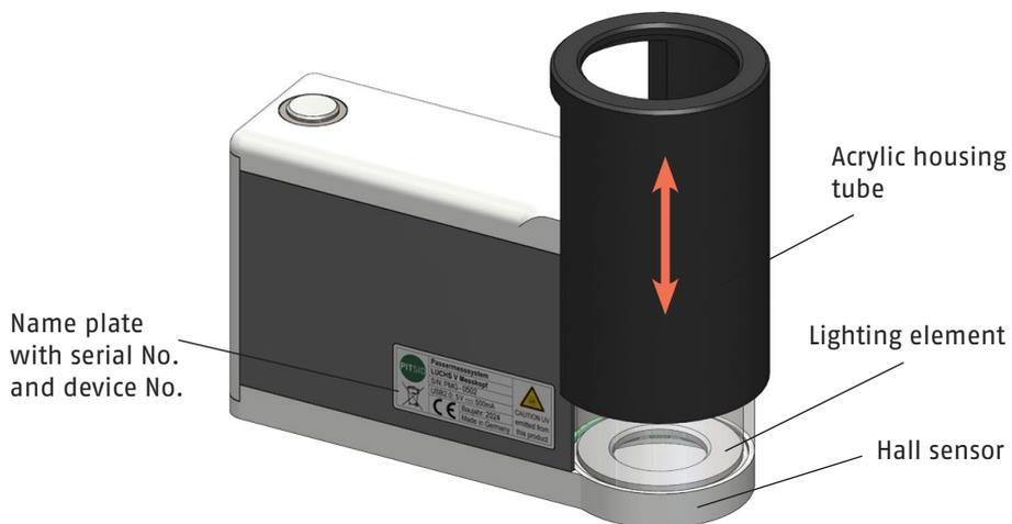
Abb. 3: LUCHS V-Measuring Head, rear view
