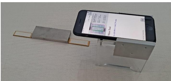
*Image 2: System for determining the dimensions and shape accuracy of large flat objects*
