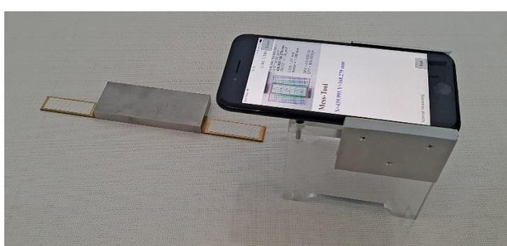
*Image 2: System for determining the dimensions and shape accuracy of large flat objects*
