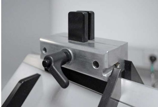
Bild 2: The jointly developed clamping device for holding the sample
