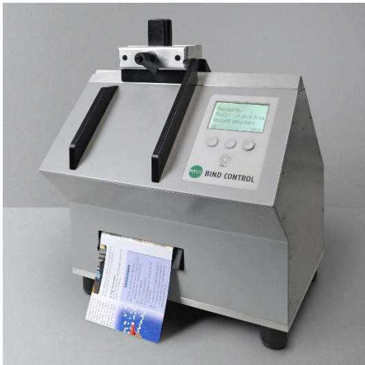
Bild 1: The Perfect Binding Tester BIND CONTROL is used by the Druckerei Vettters printing company for determining the residual strength in the fold
