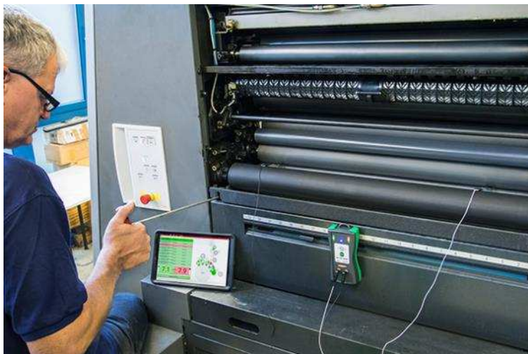
Image 2: Simple adjustment of the nip width with immediate display of the actual measured values
