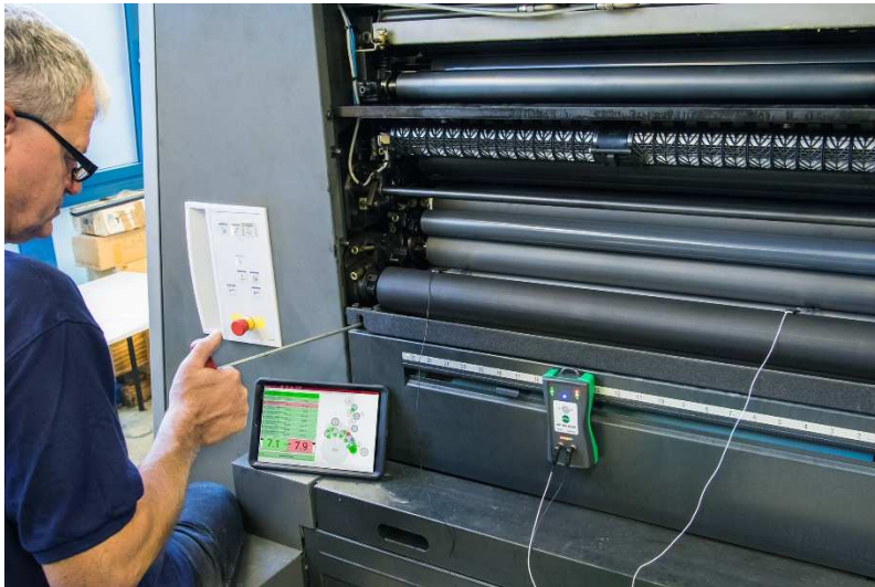
Image 1: An example from the extensive PITSID portfolio: The NIP CON SMART for fast and precise adjustment of the contact nip in offset presses.
