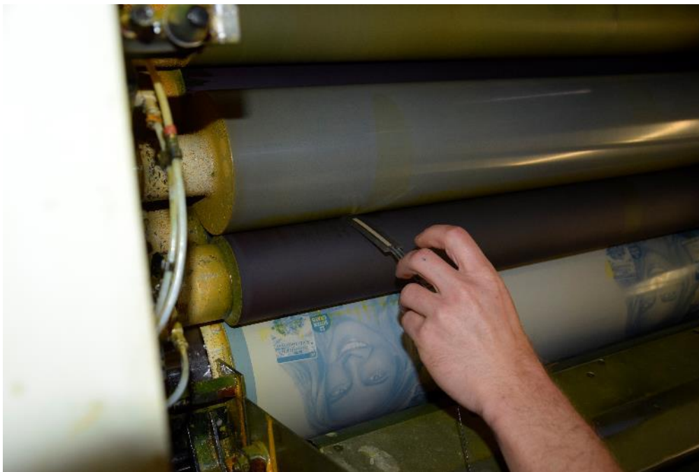
Image 1: Inserting the easy-to-handle sensors for contact zone measurement
