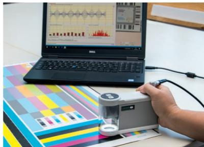
The LUCHS Register Measuring System is today used worldwide for the quality control, adjustment and error analysis of printing presses. It is able to measure the transfer, front-to-back and feed register of multicolour printing presses. Optionally, the device can be used to measure the varnish, the folding and cutting register. The measurement is carried out by recording and analysing special measuring elements located at different positions on the printed sheet.
