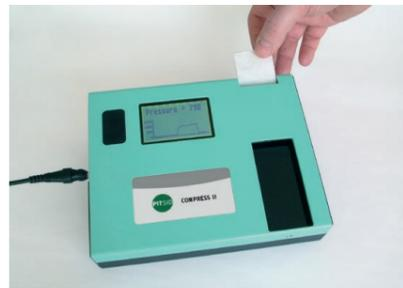
The Contact Pressure Tester COMPRESS II has successfully proven itself to be irreplaceable during printing press assembly and service. It allows for the control of the contact pressure between the bearer rings of printing presses by comparing the calculated actual value to a predetermined set-point value.
