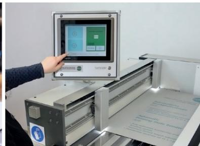
With the automatic printing plate bender APB, it is possible to bend a printing plate while referencing the position of the printing form independent of any format variations of the plate itself. In this way, a precise and axially parallel printing image position is achieved after mounting on the sleeve or plate cylinder.
