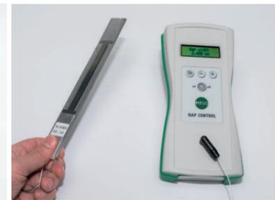
The Gap Gauge GAP CONTROL is a technical innovation which makes everyday tasks during machine assembly easier. The GAP CONTROL has been developed in order to precisely determine typical gaps starting at 1.8 mm between hard pairs of rollers or cylinders. At the same time, the device is able to determine the width between slots or slits in mechanical components.
