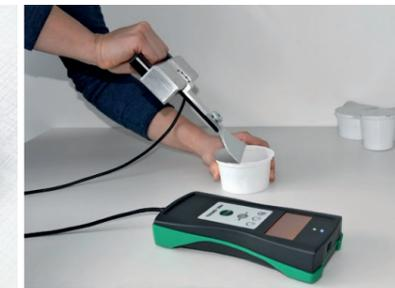
The Separating Force Gauge PEEL CONTROL is intended to measure the opening force of peelable, seam-sealed packaging or the separating force of materials that have been glued, heat sealed or laminated together.
