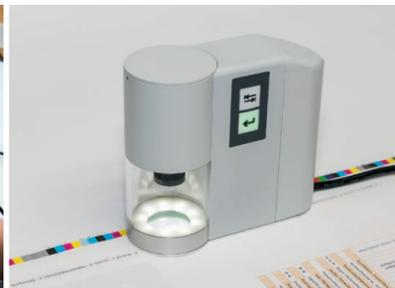
The Register Measuring Process makes it possible to carry out highly precise measurements in sheet-fed offset printing with practically invisible coded micro-marks either inline or offline. The measuring marks can even be placed inside narrow print control bars.
