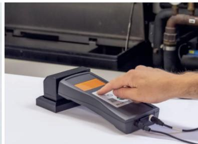
The hand-held IPA measuring device makes it possible to determine the exact alcohol concentration in the dampening solution quickly, easily and very precisely. Dampening solution samples can be taken at any point in the dampening solution circulation.
