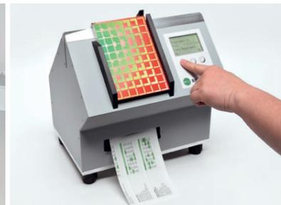
The Perfect Binding Tester BIND CONTROL is intended to measure and quantifiably evaluate the pull-out strength of single pages from a book block. It is the first device that measures a trimmed book block of a uniform width.
