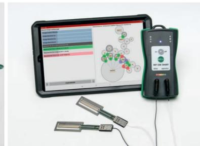
The Contact Zone Gauge NIP CON SMART is used to precisely determine the contact zone width (NIP width or contact pressure) between elastic and hard rollers. It is therefore ideal for checking and correcting the setting of dampening rollers and inking rollers in printing presses. The device can also be used for corresponding paired rollers in other processing machines.
